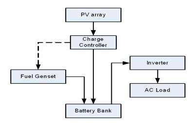
Figure 1. Block diagram of HSAPV system
