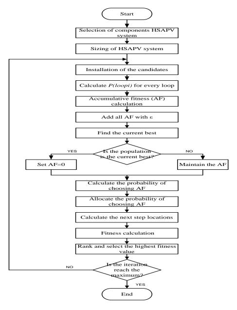
Figure 2. Flowchart of Sizing and optimization technique using DEA
